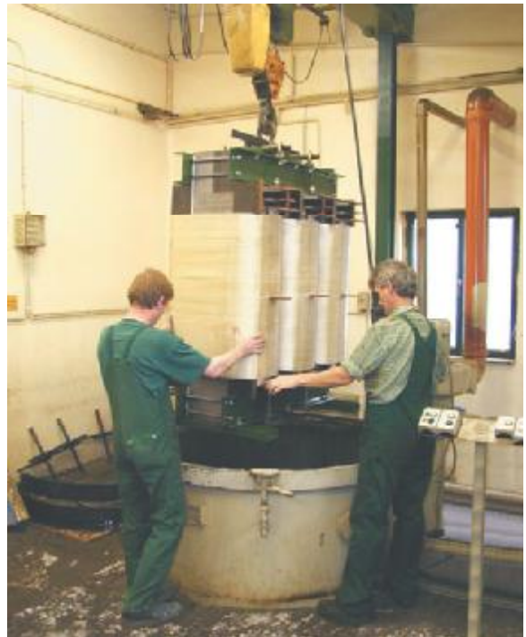
Fig. 9: Vacuum/overpressure impregnation equipment
