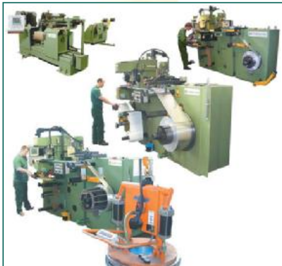
Fig. 8: Computer controlled winding machines
