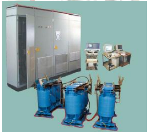
Fig. 5: Harmonic generator for real load tests
