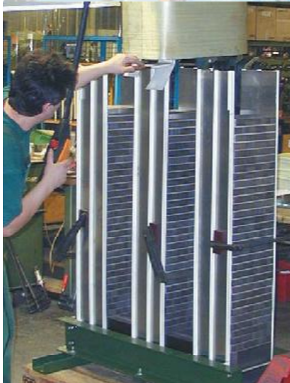
Fig. 4: Assembly of a three phase iron cored reactor
